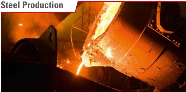
Oxygen, nitrogen and hydrogen can affect the steel properties immensely.
